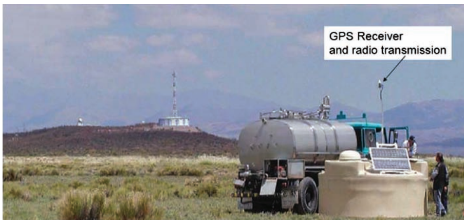
FIGURE 11.6 View of Auger South, with a surface detector tank in the foreground and a fluorescence telescope in the background. (Courtesy of the Pierre Auger Observatory.)
