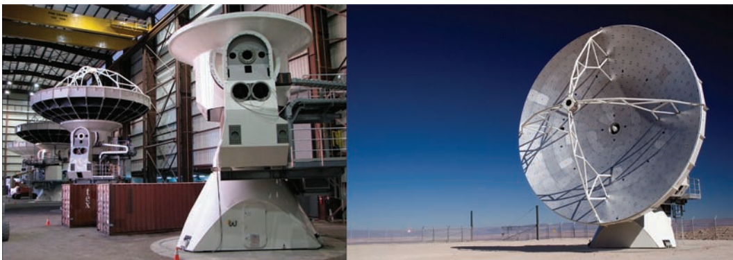
FIGURE 12.9 ALMA Vertex telescopes at various stages of assembly at the Operations Support Facilities. (From © ALMA (ESO/NAOJ/NRAO).)
